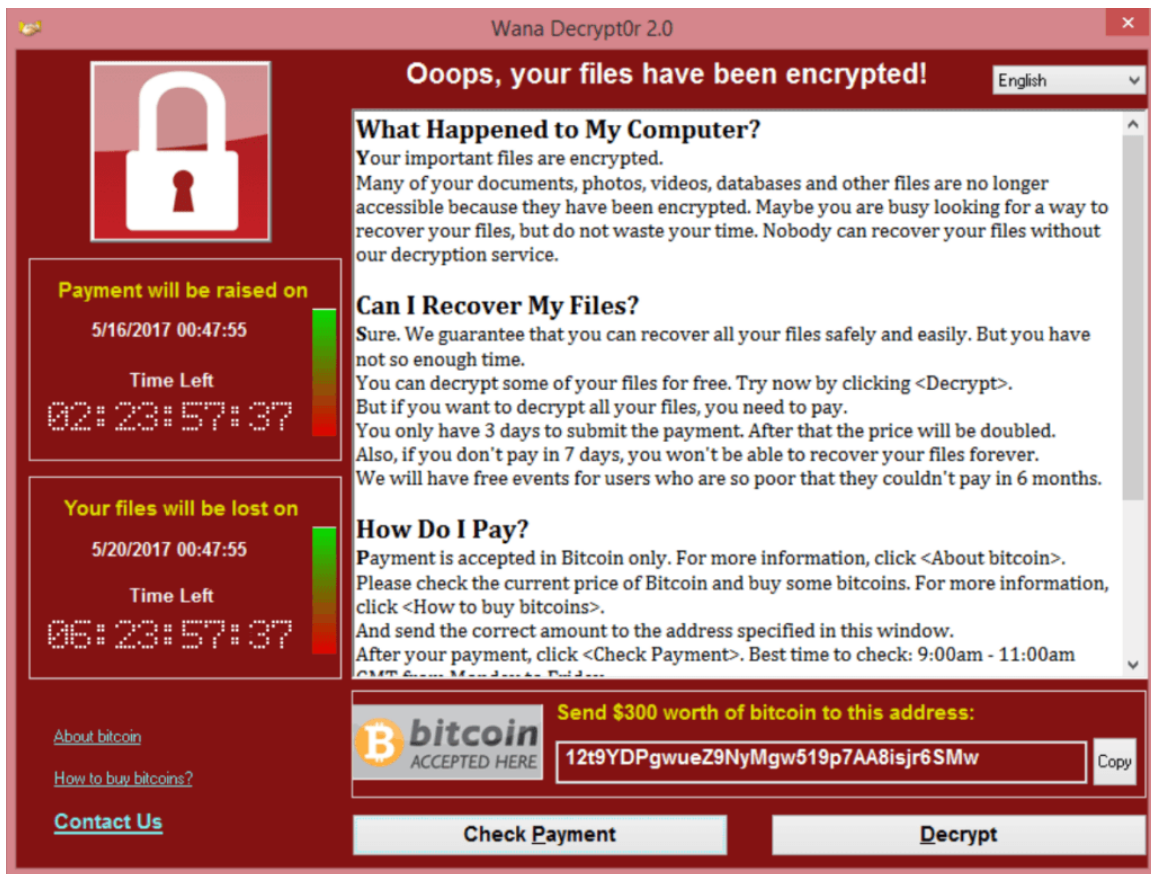
Figure 2-2: This screenshot shows the prompt shown after the WannaCry ransomware has finished encryption of the whole hard disk. The attack uses a bug in the OS to compromise the whole system. It then encrypts the hard disk, sends the decryption keys to the attackers and then deletes those keys from the local system. The only way to recover the keys is by paying the attacker $300 via Bitcoin and hoping to re-obtain the decryption keys.
