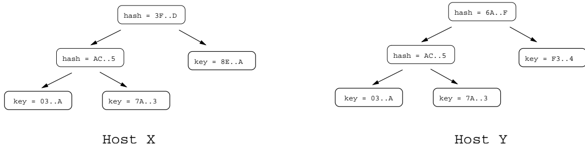
Figure 4-1: Simplified database indexes for two hosts X and Y .
